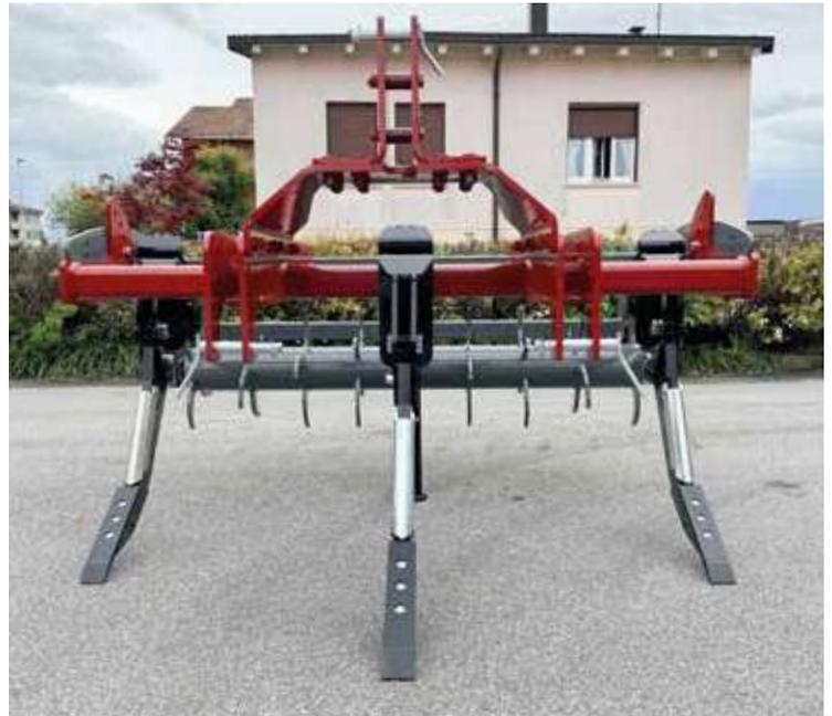
*The subsoiler Rambo Medium is a model suitable for working with tractors from 60 to 125 HP.*
