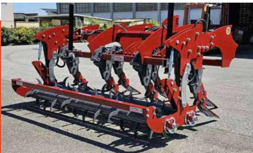
*The machine works from 150 to 280 HP tractors and is produced with frames from 2,50 to 4,00 meters. The new subsoiler RAPTOR, an evolution of the old CHD Hercules Mega, is ultra reinforced and has a totally welded frame.*
