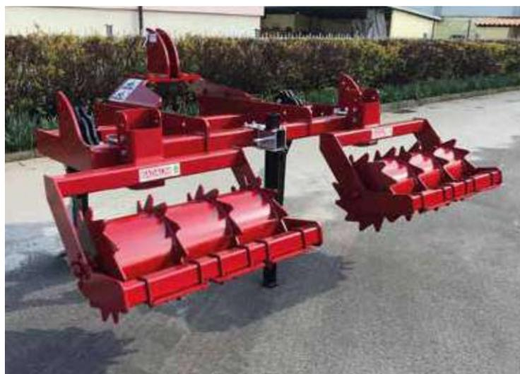
*The Badalini CMS is a small subsoiler ideal for draining in tomatoes and vineyards. The use of the CMS makes it possible to create an optimal substrate for crops while achieving conditions that limit erosive and polluting phenomena, as well as allowing rational use of natural water resources (groundwater inputs, precipitation). The subsoiler is made with a frame of 2,00 or 2,50 meter and with back rollers of 60 or 80 cm.*
