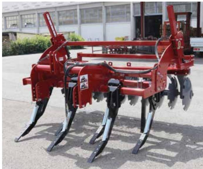
*This model is suitable for tractors from 60 to 125 HP and is equipped with breakaway safety bolts, wear guards and an interchangeable hardened chisel. It can work at a depth of 30 to 60 cm.*
